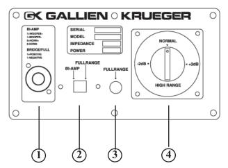
1) **Speakon® Connector:** A high current speaker connector. Use the provided 4-conductor Speakon® cable for Horn Bi-Amp operation. Pins 1+ and 1- connect the main amplifier to the woofers. Pins 2+ and 2-, connect the horn amplifier to the tweeter. You may use a standard 2-conductor Speakon® cable for full range operation.
